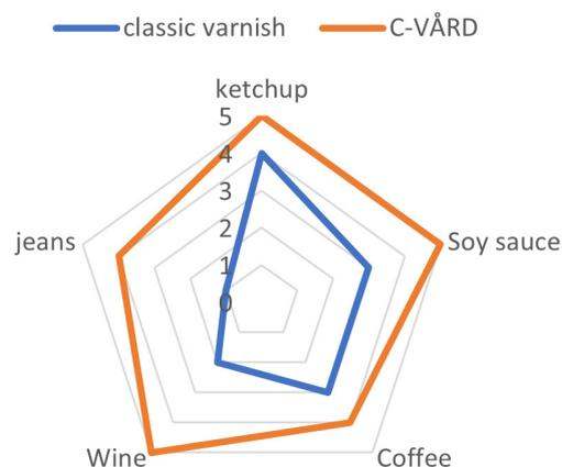
**Test method** : The samples are rubbed 10 times with impregnated cloths. After 3 hours, the test tube is cleaned with a soft brush and soap, rinsed and wiped with a cotton cloth.
